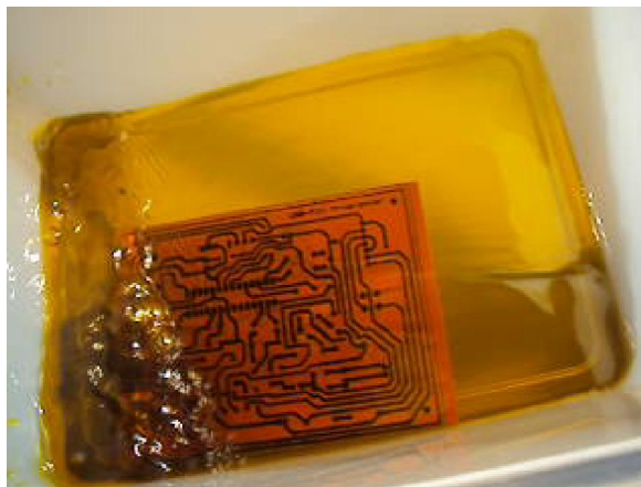
Figure 3.33 The container is agitated until unwanted copper is removed
