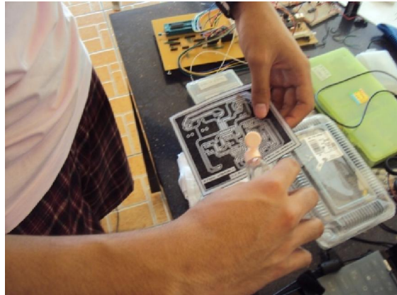
Figure 3.30 Applying oil to printed layout for transparency
