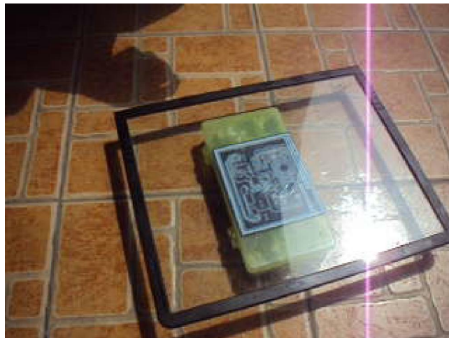
Figure 3.31 Exposing the PCB to sunlight
