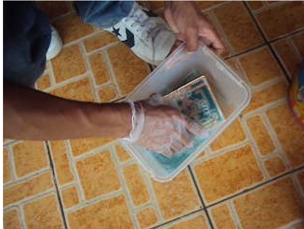
Figure 3.32 Immersion of board layout to PCB developer
