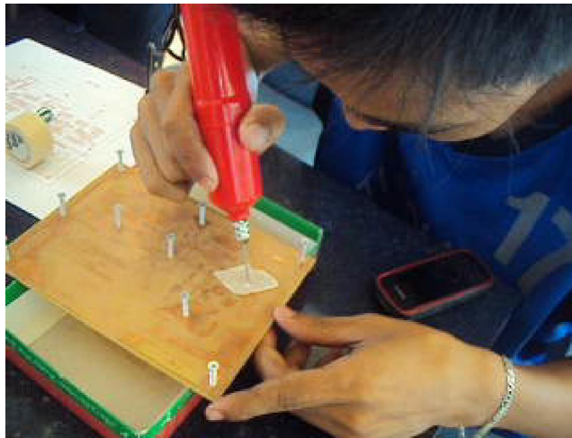
Figure 3.34 Drilling of the holes in the board
