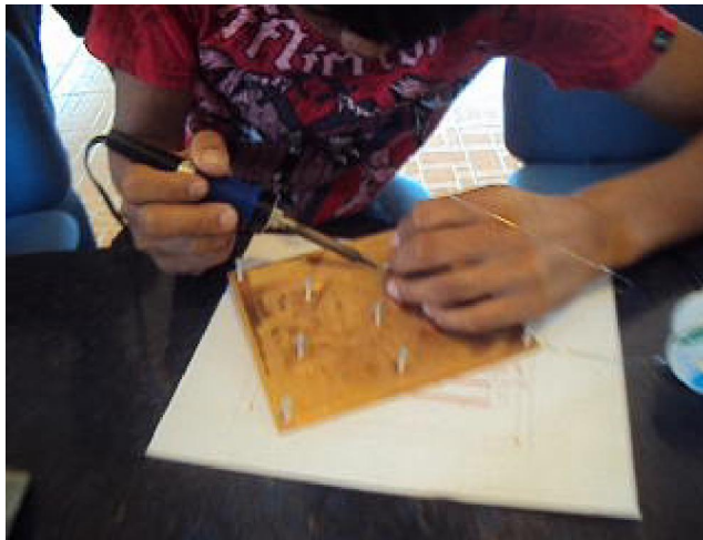
Figure 3.36 Soldering of components to the board
